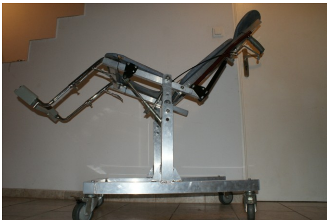
Figure 2. Engineering diploma project - bathing armchair for a handicapped person and a device for rehabilitation of scoliosis [9]
