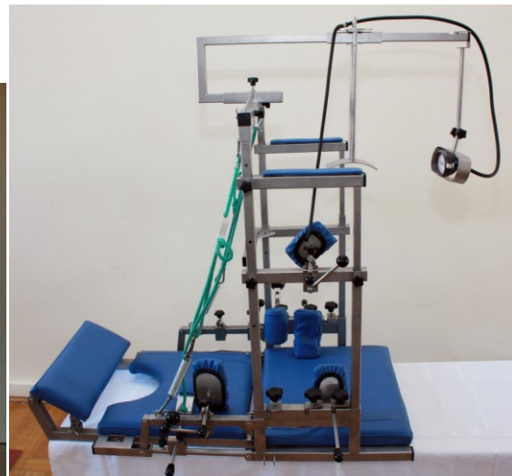
Figure 2. Engineering diploma project - bathing armchair for a handicapped person and a device for rehabilitation of scoliosis [9]
