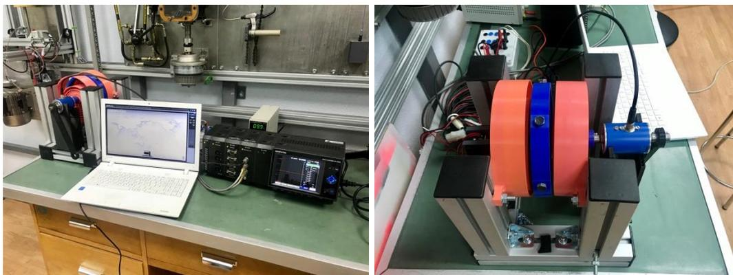
Figure 3. Prototype spring testing device.
