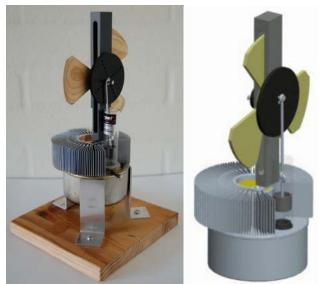
Figure 5. Example of successful engine (left) and the CAD model of the same engine (right).
