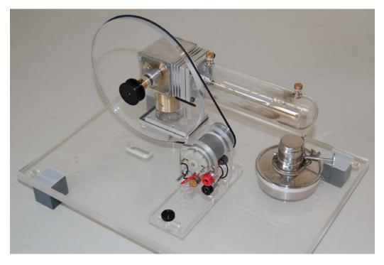
Figure 3. Transparent Stirling engine used for second assignment
